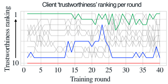
Figure 5: Client trustworthiness ranking on each round according to the Krum defence for the CIFAR-10 task. The attacker (red) is consistently ranked least trustworthy, however, we also observe some clients (e.g. the lower line coloured blue) are consistently lower ranked than others (e.g. the upper line coloured green).
